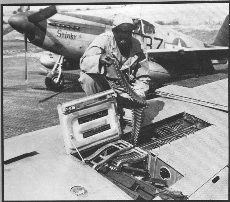
Above: Armorer re-arming a P-51 Mustang of 322nd. Fighter Group.
